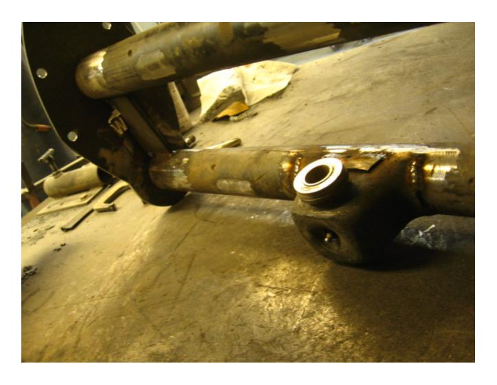
7) After the shock towers are welded on, remove it from the bus. Now you can cut the braces off. Re-weld your center pin carrier back on, postion it in the center of the lower tube. The center pin should be parallel to the beam tubes. Also notice that I welded a  $2" \times 1/4"$  gusset between the tubes on the back side of the shock towers for added strength.
