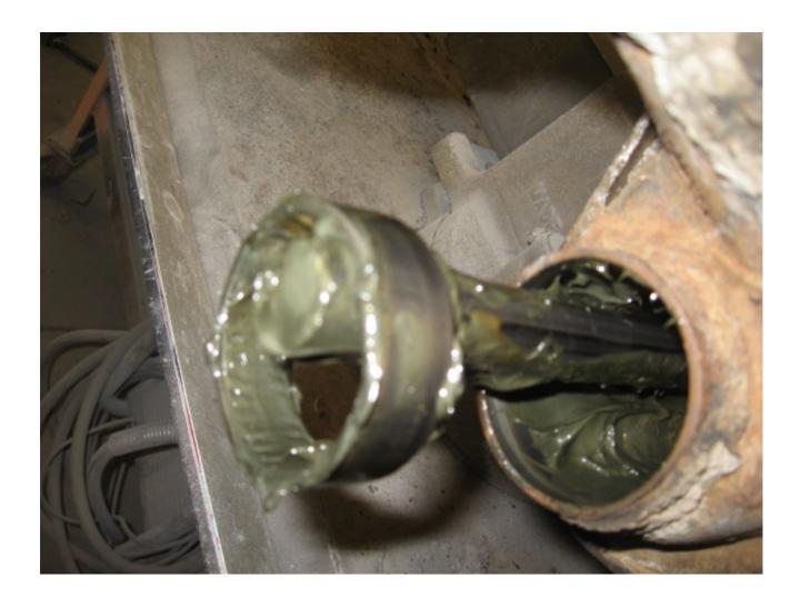
2) Once the beam is cut in half its easy to remove the dust seal cups and bearings. I like to use a piece of pipe and a hammer. I remove the bearings to prevent damage to them when I'm welding on the new shock towers. Also notice that I left the inner bearings. They are located far enough in the tubes that they are not in danger of being damaged, plus they are easy to ruin when trying to remove them.
