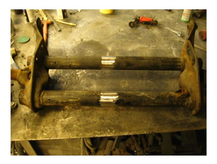
4) Be sure to slide the center block in BEFORE welding the beam back together. I like grind bevels on the ends of the tubes so that the weld will be very strong. Clamp the beam in a vice and use several C-clamps, then use a strait edge to make sure the beam tubes are strait. After the beam tubes are aligned corectly, start welding it back together. I'll weld as much as I can before removing any clamps, then I'll remove one clamp and welds as much as I can before removing another clamp.
