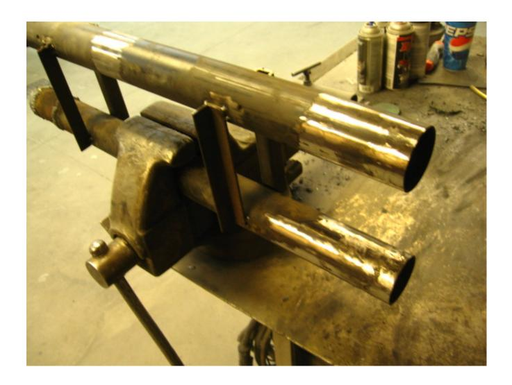
5) Since the beam was narrowed from the middle, the mounting locations on the stock shock towers will be too narrow to fit the frame on the bus. To solve this problem I have custom 1/4" plate shock towers that mimic the shape of the original shock towers. You'll have to do some measuring and cut the shock towers out of 1/4" plate.
