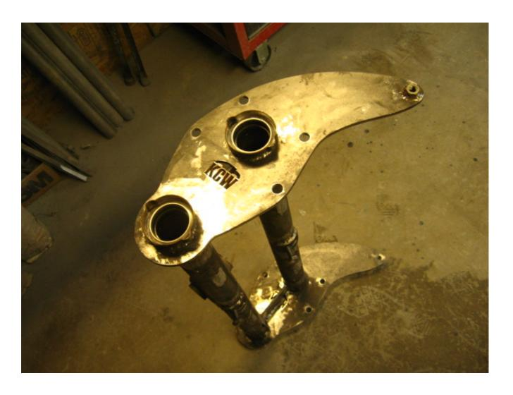
9) Now that all of the cutting and welding has been done on the beam its time to re-install the bearing and dust seal cups. All thats left now is to narrow the tie rods and torsion springs the same amount as the beam.
