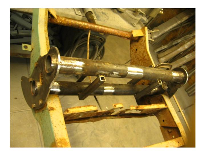
6) I have a bus frame section that I use to build bus beams. I'm guessing that most of you won't. So, you'll have to do this step in the bus. Bolt your custom 1/4" plate towers to the bus and center your beam between them. Do as much welding as you can with it bolted in the bus to keep things from twisting/warping.
