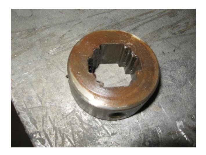
3) Remove the center block from the old tube sections. I like to carefully cut a slit in the tube and pry it apart so that the block will simply fall out. Next, make sure that the center block will easily slide into the regular beam tube, you may have to remove a little material from the O.D. with a belt sander. If the center block is tight in the beam tube, it will be hard to adjust later.
